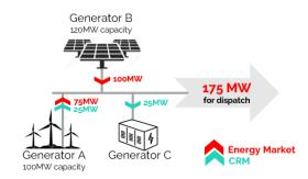
CRM allows Gen A to put an additional 25MW into the grid by **trading** additional capacity behind the constraint in the CRM. It also enables Gen C to charge (place a load). Enabling an additional 25MWh into the grid
