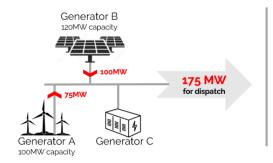
Both generators are constrained, resulting in **only 175MW of the available 220MW able to be dispatched**, resulting in underutilisation and spilled energy.
