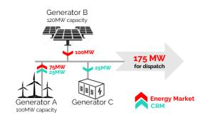
CRM allows Gen A to put an additional 25MW into the grid by **trading** additional capacity behind the constraint in the CRM. It also enables Gen C to charge (place a load). Enabling an additional 25MWh into the grid
